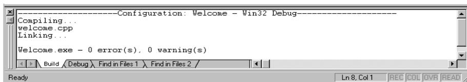
Fig. 1.11 **Output** pane showing a successful build.
