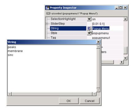
**Determining Which Item Is Selected.** The Value property contains the index of the selected item. For example, if the String contains the three items, peaks, membrane, and sinc and the Value property has a value of 2, then the item selected is membrane.
