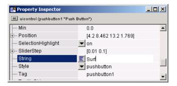
You can view the change by clicking the Layout Editor. Similarly, change the String property of the middle push button to Mesh, the bottom push button to Contour, and the Static Text to Select Data.
