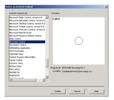
**3** Click **Create** to display the ActiveX control in the Layout Editor, and resize the control to approximately the size of the square shown in the preview pane. You can do this by clicking and dragging a corner of the control, as shown in the following figure.
