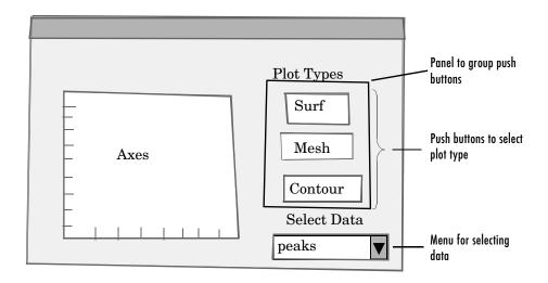
A panel contains three push buttons that enable you to select the type of plot you want. The pop-up menu contains three strings — peaks, membrane, and sinc, which correspond to MATLAB functions. You can select the data to plot from this menu.
