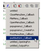
Clicking a callback on the list displays the section of the M-file containing the callback, where you can edit it. This example shows the callback template for pushbutton1\_Callback.
