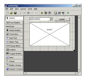
When you run the GUI by clicking the Run icon  $\triangleright$  on the toolbar, the GUI displays a plot of five random numbers generated by the MATLAB rand(5) command, as shown in the following figure.
