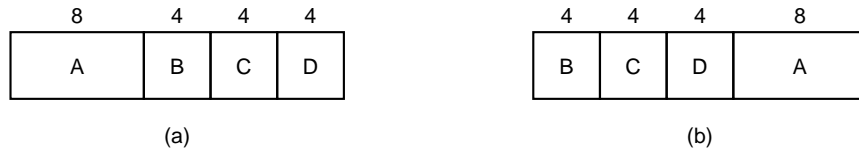
Figure 2: An example of shortest job first scheduling. (a) Running four jobs in the original order. (b) Running them in shortest job first order.
