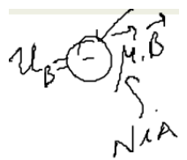
Fig. 28-21 A side view of a circular coil carrying a current and oriented so that its magnetic dipole moment is aligned with magnetic field \vec{B} .
