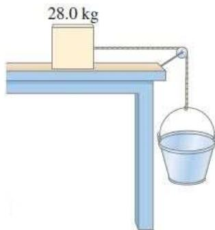
The coefficient of static friction between the table and the block is 0.45 and the coefficient of kinetic friction between the table and the block is 0.32. Sand is gradually added to the bucket until the system just begins to move.
