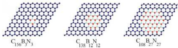
Figure 2. Optimized geometries for Xh-BN(H)@G hybrid nanosheets (see Table 4). Dark blue, light blue, and red colors respectively show C, B, and N atoms.
